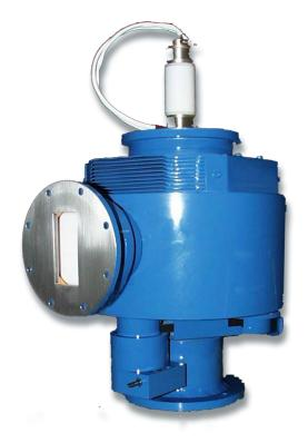
A magnetron is a high power microwave oscillator in which the potential energy of an electron cloud near the cathode is converted into RF energy in a series of cavity resonators. The VMS1197B magnetron delivers high peak and average RF power for use in medical or industrial applications.
